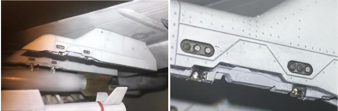
The opposing magnet goes on the rail. In this case I Close up shot of the magnets CA'd into the slot. didn't have to drill a hole to get the correct gap between the rail and the ordnance. If needed you can drill a small 1/32" diameter hole for the magnet.
